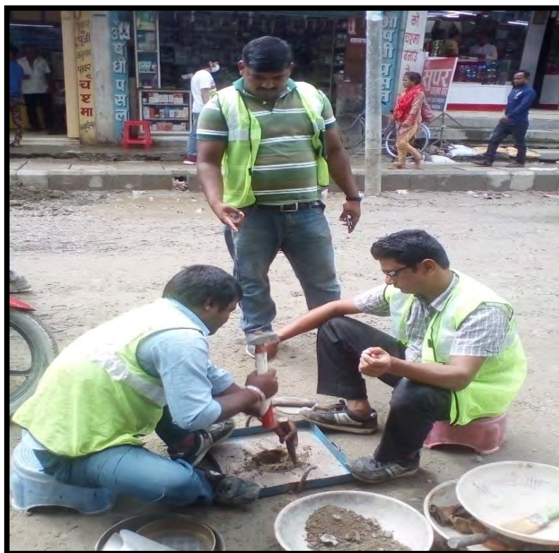
Field density test – Sand replacement method for sub base
