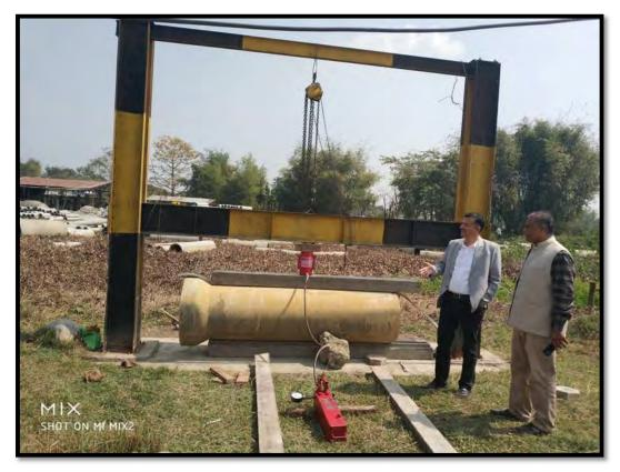
Three edge Bearing test of Hume/RCC Pipe
