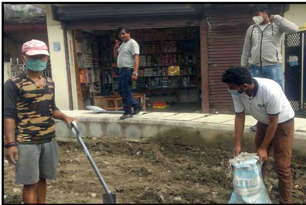
Sampling for MDD and OMC at T1Line7B
