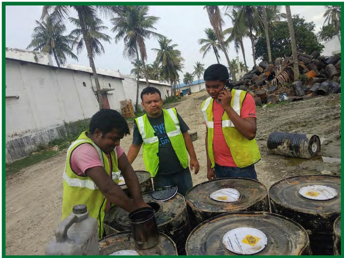
Joint sampling of Bitumen at Asphalt plant
