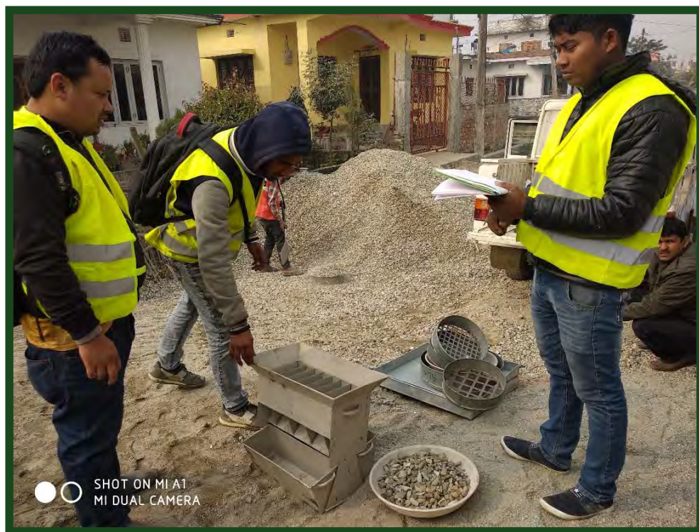
Gradation check of M20 aggregates at site
