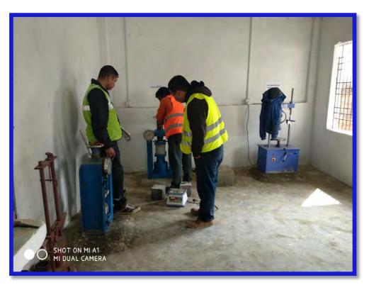
Cube crushing at Laboratory
