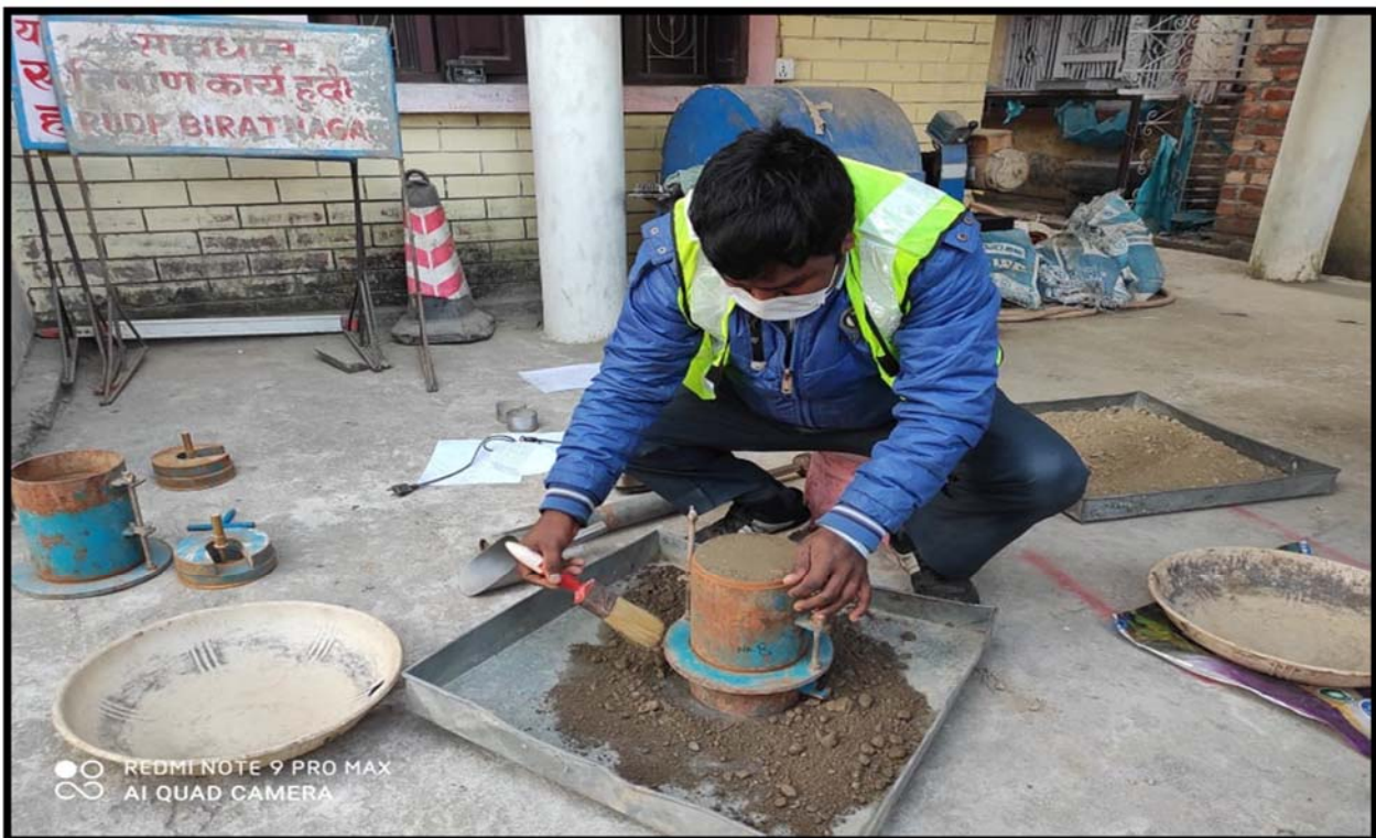
Moulding for CBR of Subbase at Lab
