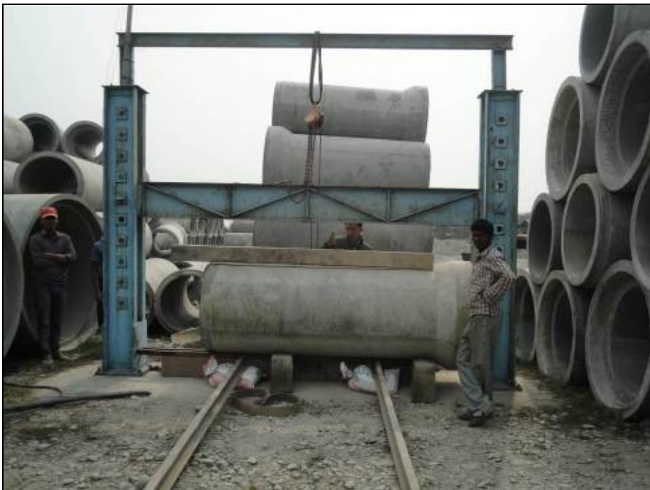
Three Edge Bearing Tests of RCC at Hume Pipe Factory at Itahari
