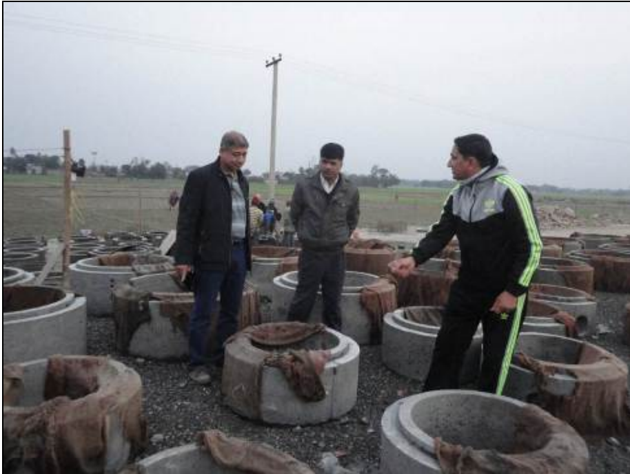
Inspection of Precast Manholes, Sewer Inlets and House Connction Chambers During Site visit of Mr Parag Kayastha, Project Dy.Director
