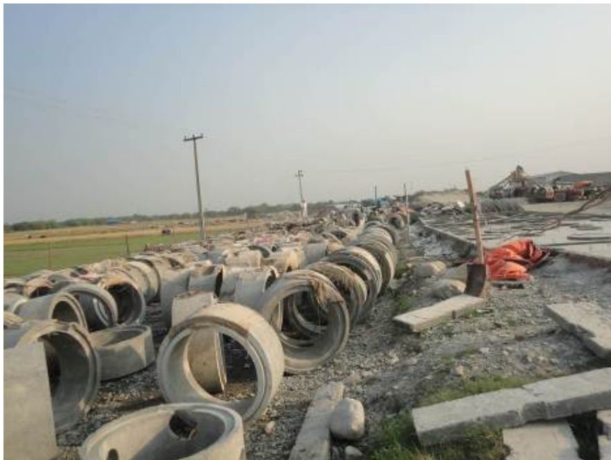
Pre-cast units in progress at Contractor's yard, Judi Katahari
