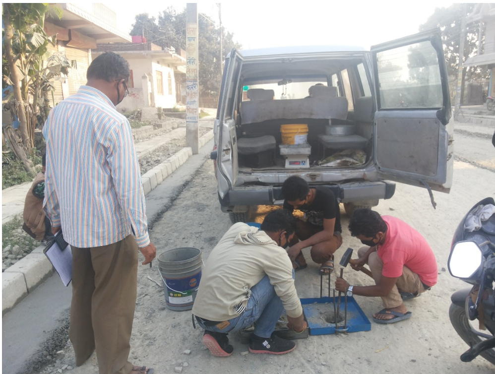
Field density test of base course at R2 Road
