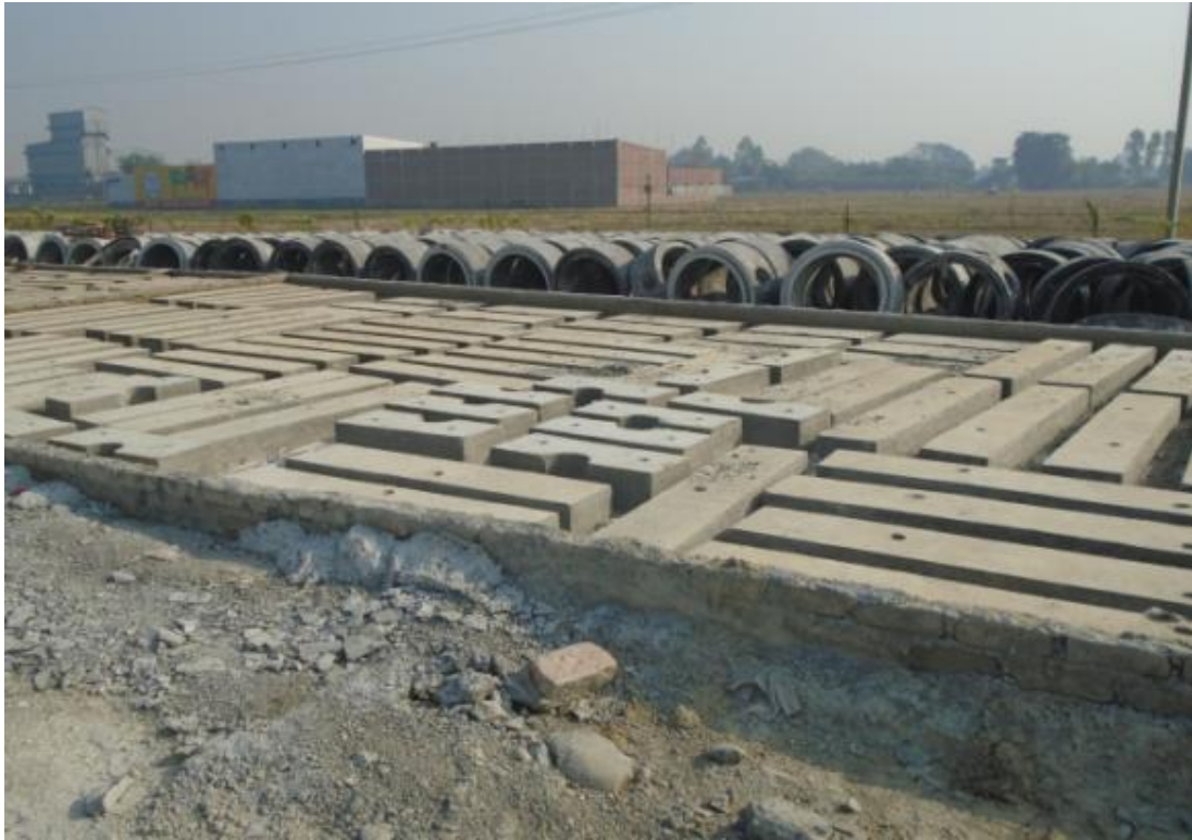
Figure 1 Precast element of Manhole/House Connection Chamber /Sewer Inlet/Drain Cover Slab Stock at Yard
